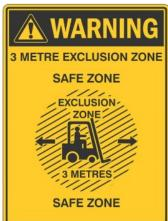
Mobile plant operators who see a person approaching must take immediate steps to ensure the mobile plant is safely brought to a complete stop, with gears in neutral and the parking brake applied, before allowing the person to enter within the 3-metre separation distance
