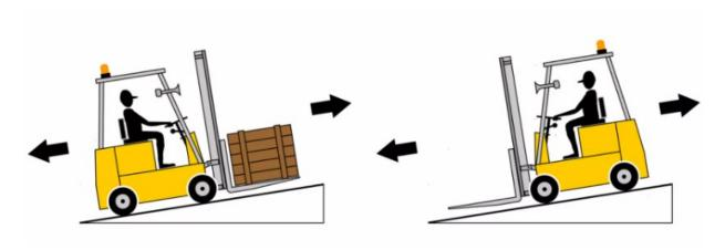
When loaded, all ways drive up or down slopes with fork pointing towards the highest part of the slope.
