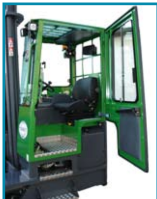
Wider Cab for increased Operator Comfort
