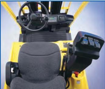
Increased productivity is directly related to the ergonomically designed operator's compartment. On-demand power steering, increased legroom and easier entry and exit make any load easier to handle. (Truck shown with optional TouchPoint<sup>™</sup> electrohydraulic mini-levers.)
