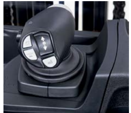
New joystick with integrated controls.
