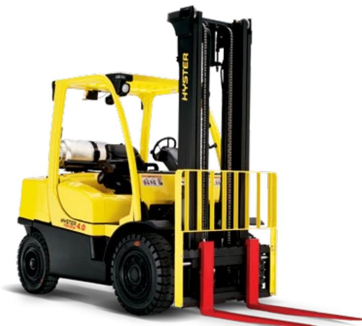
The transmissions are compatible with the combi-cooler radiator and a superior counterweight tunnel design coupled with a "pusher" type fan, to provide the industry's best cooling.
